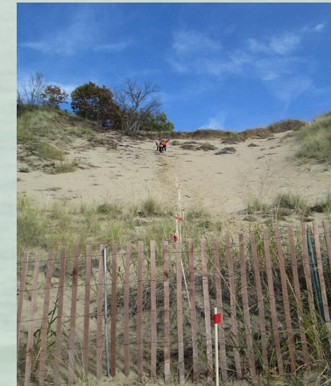
Figure 3: Researchers use erosion pins and flags to create a transect line.
