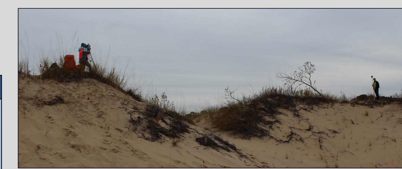
Figure 3: For the topographic survey, the total station was set up on the dune crest.
