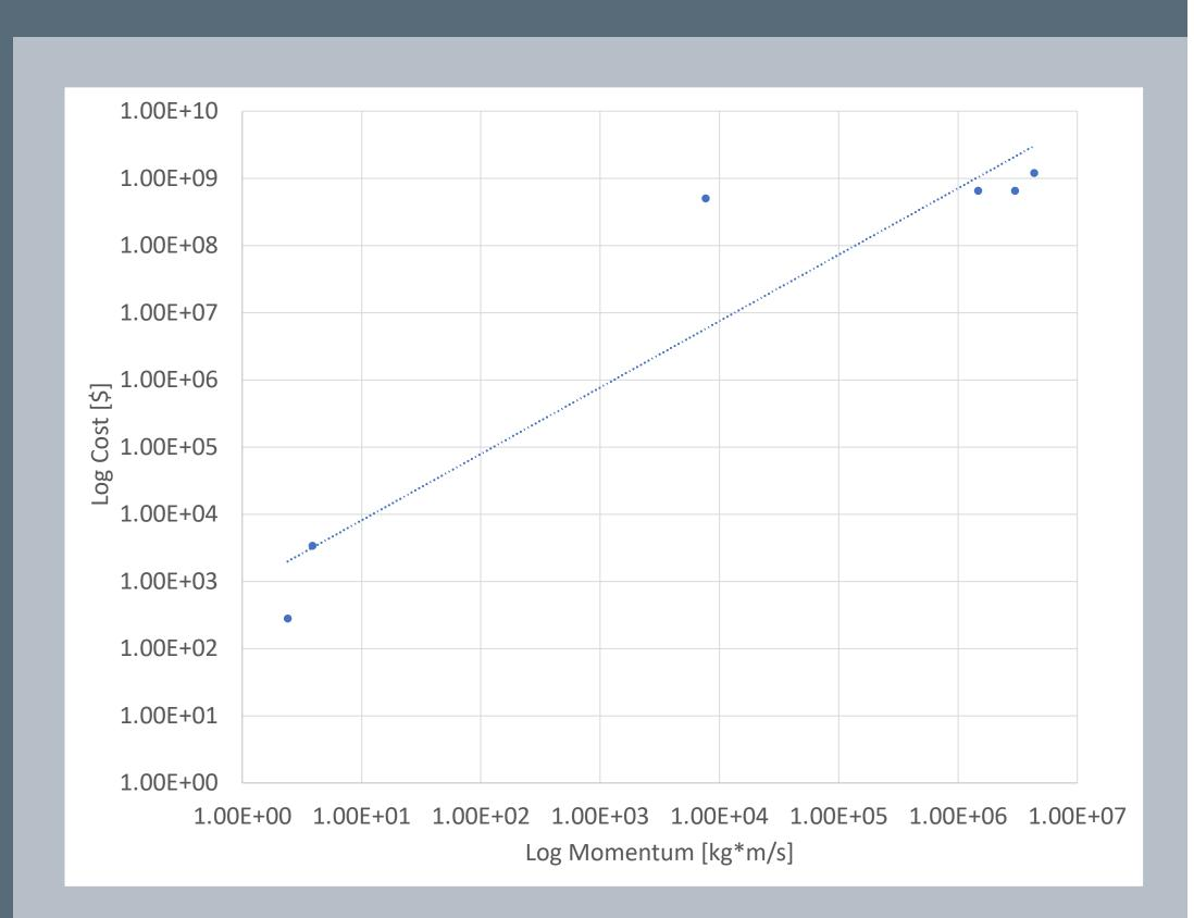
The cost model generated show a power model regression, so as required momentum increases, the cost of the linear motor and related infrastructure increases significantly.
